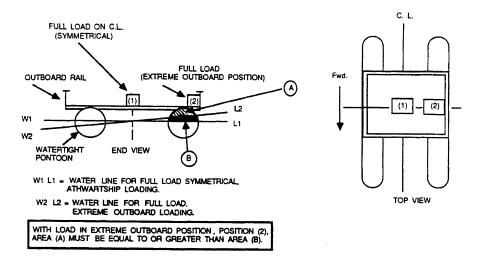
(2) With the simulated load located on the centerline at the extreme fore or aft end of the deck, whichever position is further from the initial position of the load, the top of the pontoon must not be submerged at any location, as indicated in Figure 178.340(d)(2).
