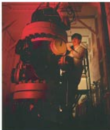
This chamber, which simulates ocean depths of 600 meters, is being used by Stephen Rowland (pictured here) to test the feasibility of disposing of carbon dioxide in the ocean. (Photo by Bob Chinn, University of Hawaii)
