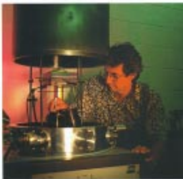
Richard Bochenko adjusts a thin-film electrolyzing device that is an important test in his efforts to design low-cost electrodes that efficiently electrolyze water into hydrogen and oxygen. (Photo by Bob Chinn, University Relations)
