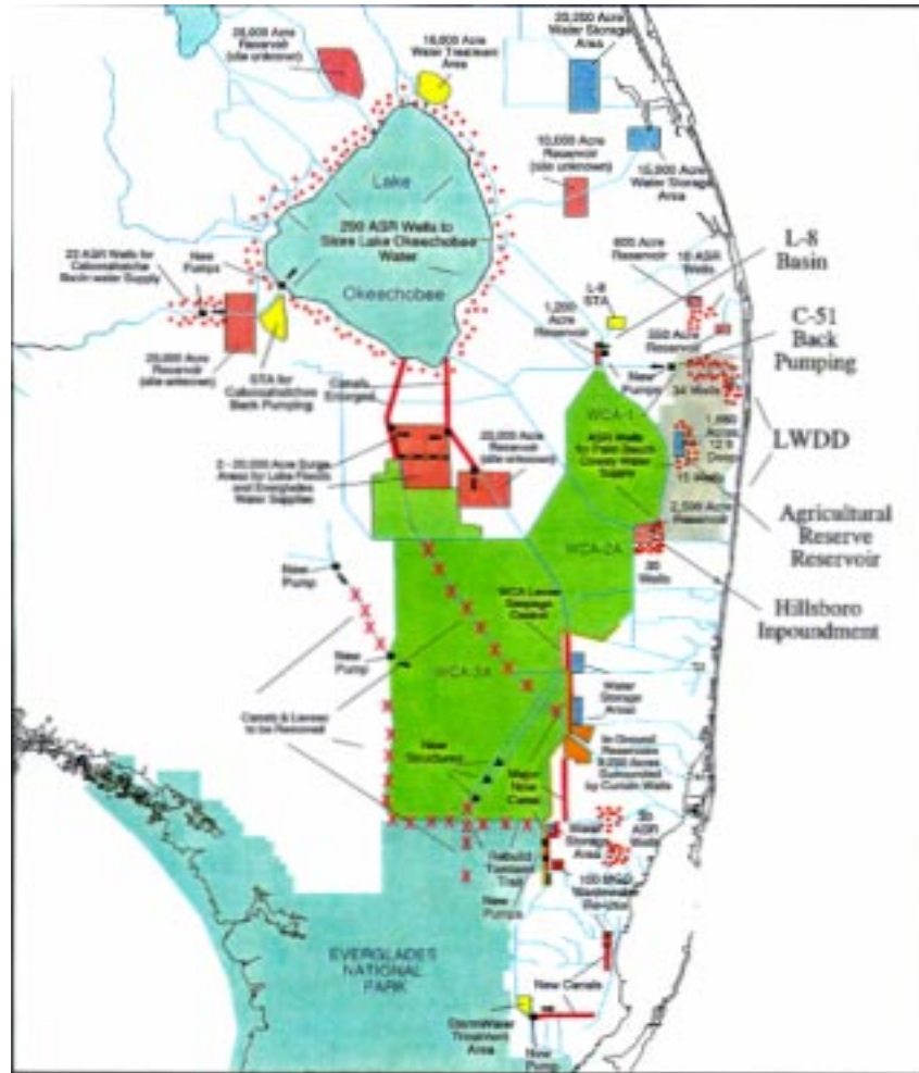
Figure 4. Conceptual diagram of the major features of the Recommended Plan in the Restudy.
