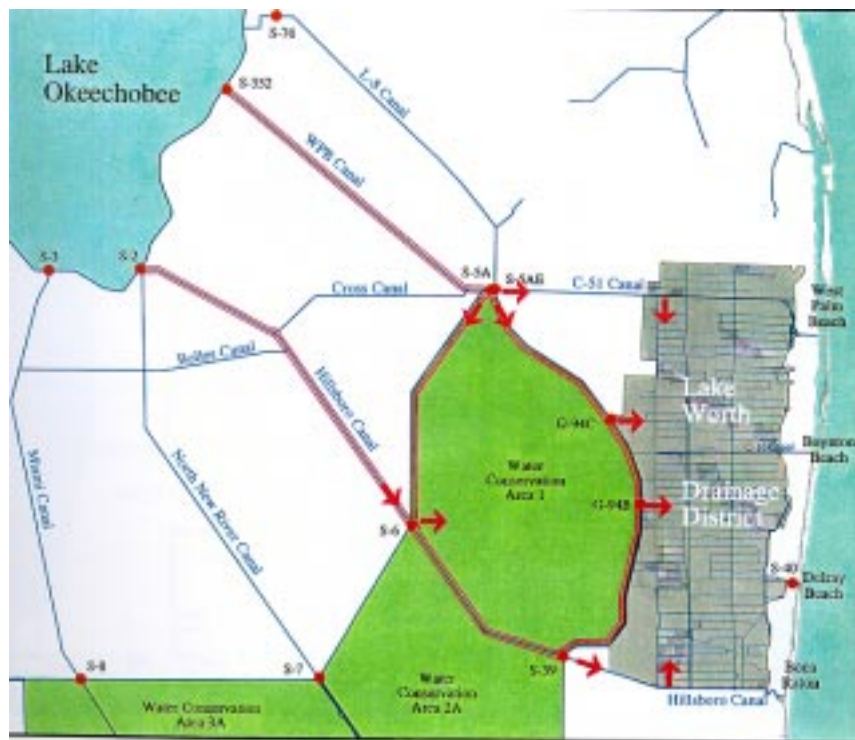
Figure 2. Connection of the Lake Worth Drainage Facilities to the federal project facilities constructed in the 1950s. The District recharges urban water supply wells in Palm Beach County by receiving water from Water Conservation Area 1 and Lake Okeechobee during dry periods.
