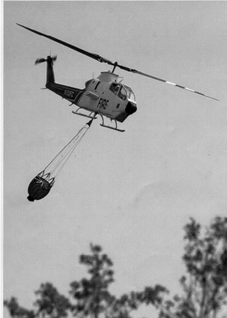
The aircraft is a demilitarized US Army AH-1F "Cobra" attack helicopter converted for forest fire fighting. The cost to the state for the conversion was approximately $300,000 as compared to a cost of $2,000,000 for a new aircraft of comparable capability.
