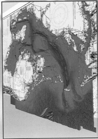
Chart illustrating the combination of USGS topographical information with bathymetric data
