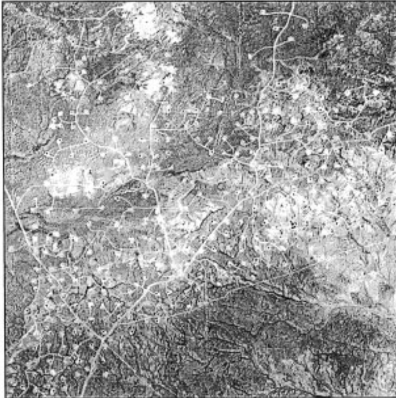
Figure 4. Landsat image taken on August 28, 2001. 40-acre spacing has been approved, and more than 300 gas wells have been drilled in the Jonah field at this point.
