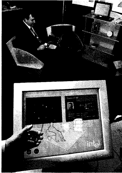
Figure 4. Sensor network with screen display. A battery-powered device wirelessly collects data from sensors embedded in household items such as a floor mat or chair. The device transmits data to the PC display to alert a caregiver about a change in a person's activity.
