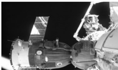
The blackness of space provides the backdrop for this scene of a Russian Soyuz TMA-4 spacecraft docked to the Station's Zarya functional cargo block nadir port in September 2004. While the Shuttle is grounded, the Russians have delivered crew and cargo to the Station. In the future, a combination of vehicles, including those provided by other international partners and commercial providers, will provide transportation to and from the Station.
