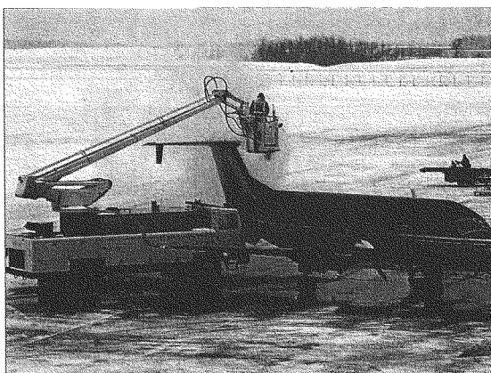
Figure 3: Example of Ground Deicing to Help Ensure Clean Aircraft
