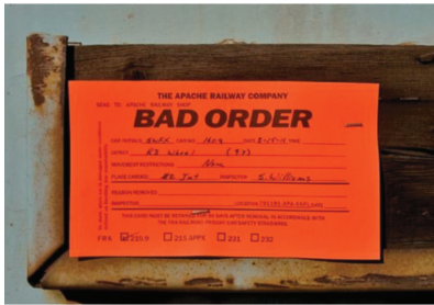
Figure 1. Example of a Bad Order tag that signifies a defect that must be fixed prior to being put back into service
