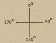
(2) The hammer and trigger orientations are obtained by rotating the pistol about the axis of the barrel, when the pistol is in the 90° or 270° orientation, so that the hammer and the trigger are each respectively closest to and in the same horizontal plane with the microphone.
