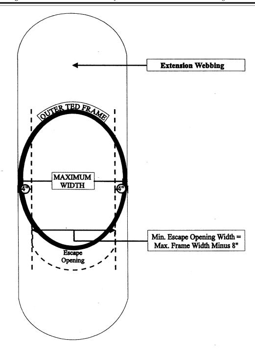
FIGURE 13 to part 227--SINGLE GRID HARD TED ESCAPE OPENING
