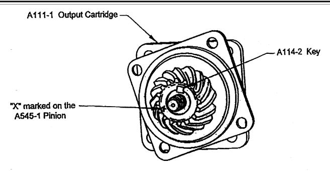
Note: The A114-1 Key for the A110-1 Input Cartridge is located similar to the A111-1 Output Cartridge depicted above
