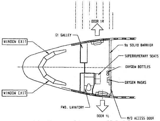
"Fig. 1: Emergency Exit Arrangement and 9g Barrier"
