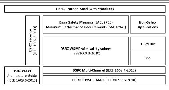
Figure III-6 DSRC Protocol Stack
