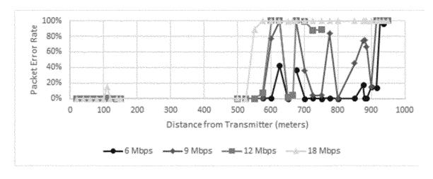
Figure III-3 Packet Error Rate based on Distance
