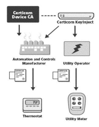
Figure V-2 ZigBee Smart Energy Certificate System
