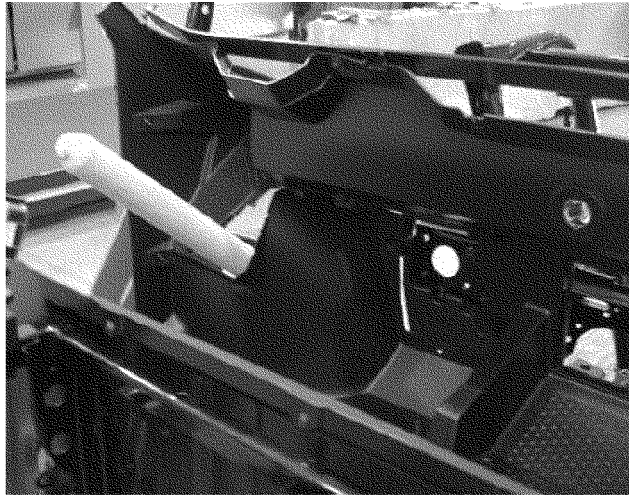
Figure 5 – Interior View, Driver's Side Floorboard Where Debris Penetration Occurred at 2.5 mph
