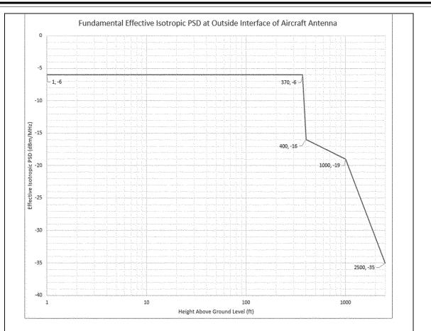
\*The notch that occurs in the curve between 370 ft AGL to 1000 ft AGL is due to the impact of the Nationwide Equivalent Isotropic Radiated Power (EIRP) Elevation Mask, 75 ft horizontal minimum separation distance (MSD), and 50 ft vertical MSD for a 5G tower at 350 ft AGL.
