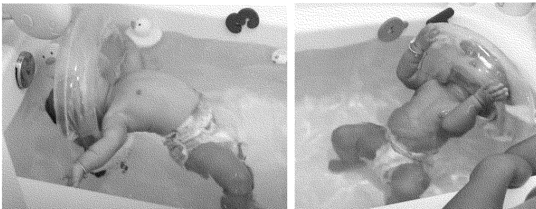
Figure 1: Children pushing up on the front underside of the neck float and leaning rearward into the discontinuous ends (partially blurred for privacy).
