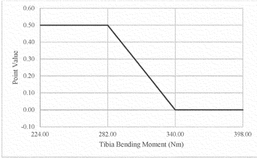
Figure 11: FlexPLI Tibia Bending Moment Scoring
