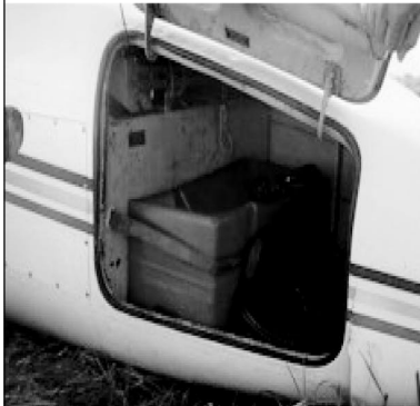
One type of illegal fuel tank installation giving aircraft extended range
