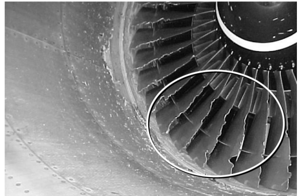
Boeing 747 fan blade damage from collision with a Western gull.
