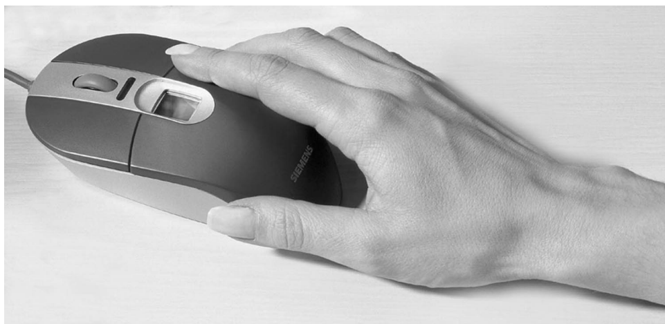
Figure 13: An Example of Fingerprint Recognition Technology Built into a Mouse
