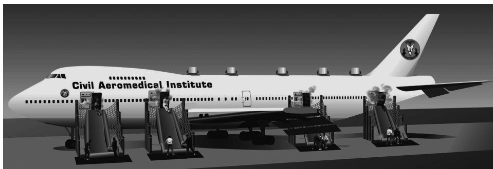
Figure 15: Drawing of Possible Emergency Slide Testing of FAA's 747 Test Aircraft
