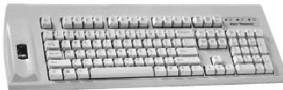
Figure 4: An Example of Fingerprint Recognition Technology Built into a Keyboard
