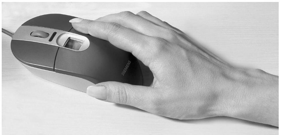
Figure 5: An Example of Fingerprint Recognition Technology Built into a Mouse
