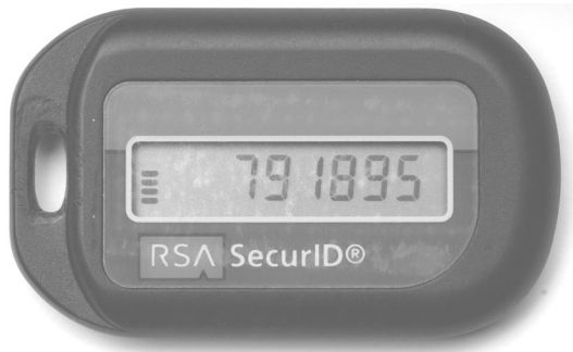
Figure 7: Example of a Time-Synchronized Token
