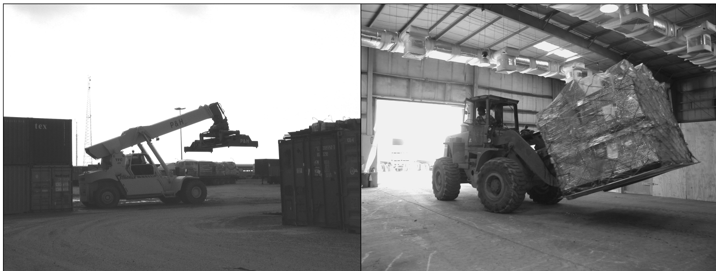
Figure 8: Rough Terrain Container Handler (left) and Rough Terrain Fork Lift (right) at the Joint Military Mail Terminal in Kuwait, December 2003
