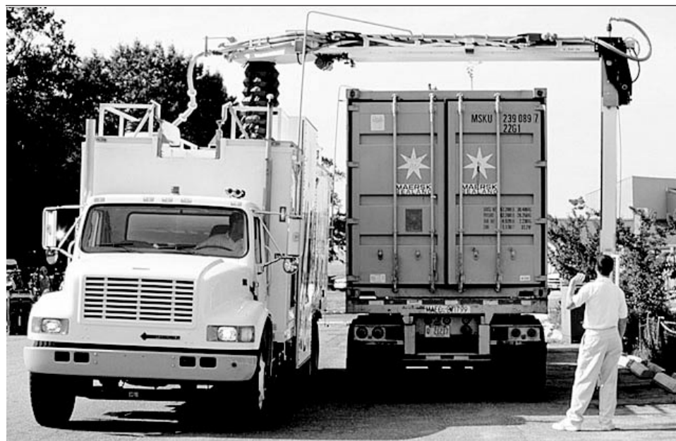
Figure 5: A Mobile Search X-ray Inspection System for Detecting Truck Bombs
