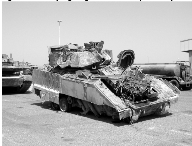
Figure 2: Bradley Fighting Vehicle—Example of Projected Equipment Item Damage
