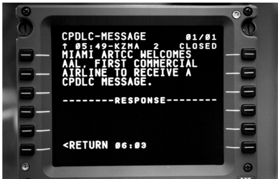
Figure 10: CPDLC Text Message on an Aircraft Display
