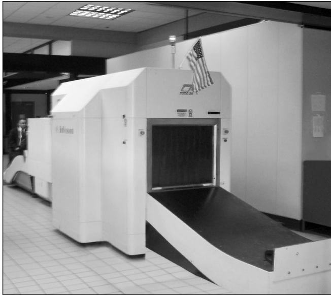
Figure 1: EDS Machine Used by TSA to Screen Checked Baggage
