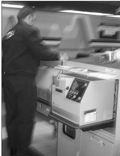
Figure 2: ETD Machine Used by TSA to Screen Checked Baggage
