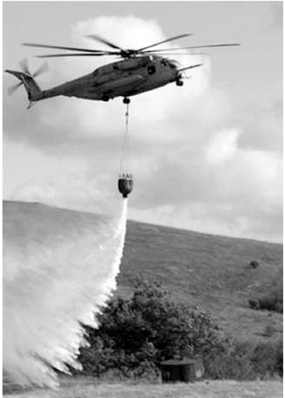
Figure 17: A Helicopter Using a Water Bucket
