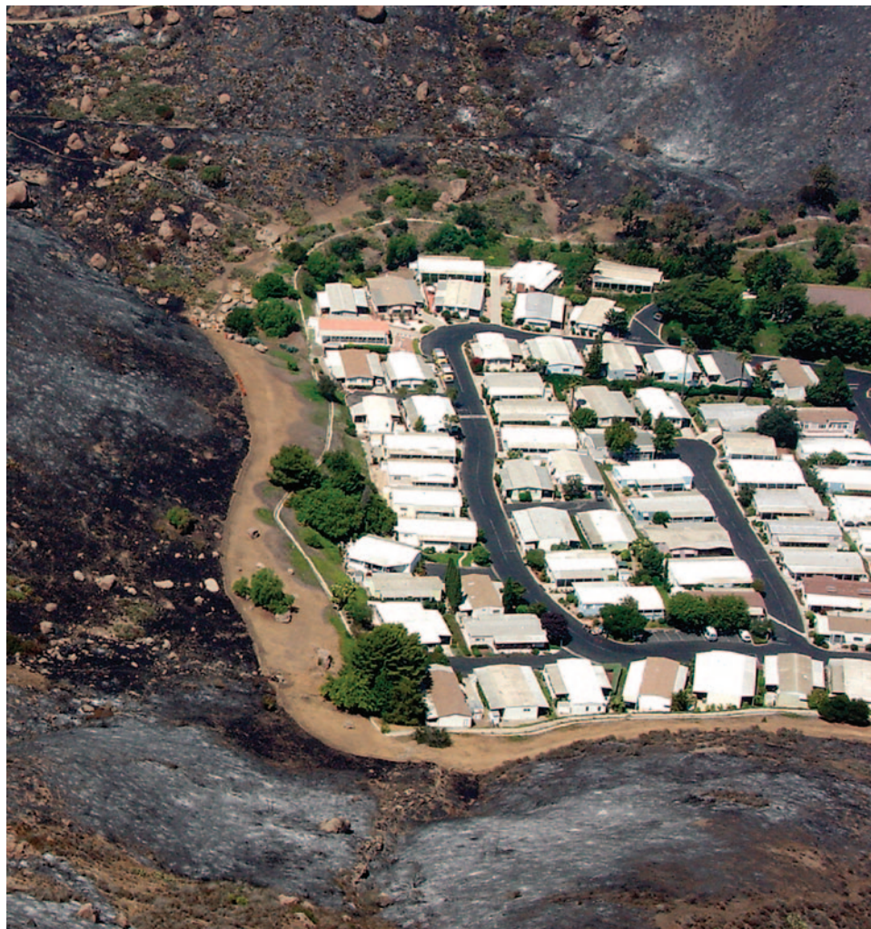
Figure 9: A California Community with Defensible Space That Survived a Wildland Fire in 2004
