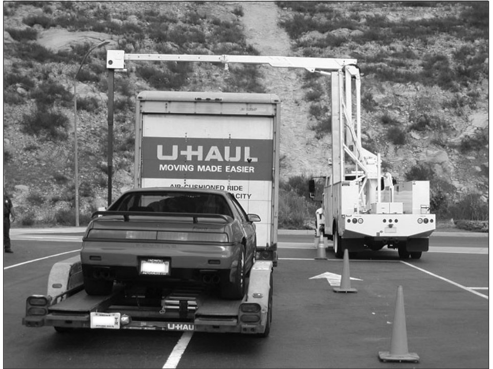
Figure 4: VACIS Machine Examining a Vehicle at the I-15 Temecula, California, Checkpoint
