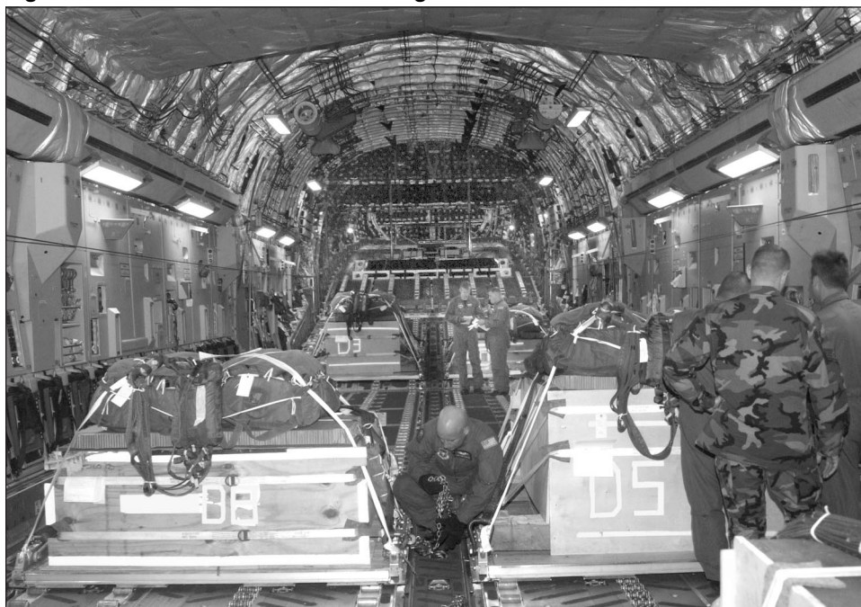
Figure 9: Loadmasters Chain Down Cargo on a C-17
