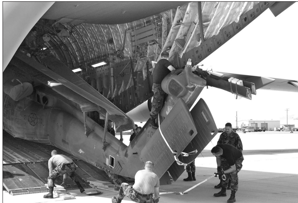
Figure 8: Unloading of a HH-60G Pave Hawk Helicopter from a C-17 in Support of OIF
