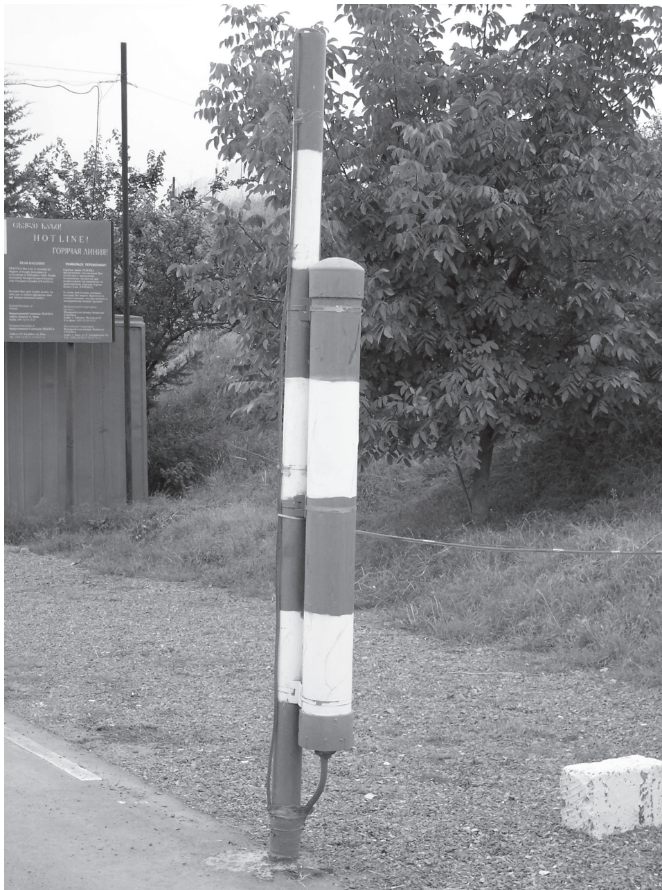
Figure 2: Older Radiation Portal Monitor Able to Detect Only Gamma Radiation at a Border Site in Georgia
