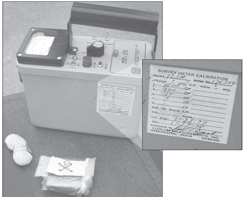
Figure 3: Handheld Radiation Detector in Georgia Needing Recalibration
