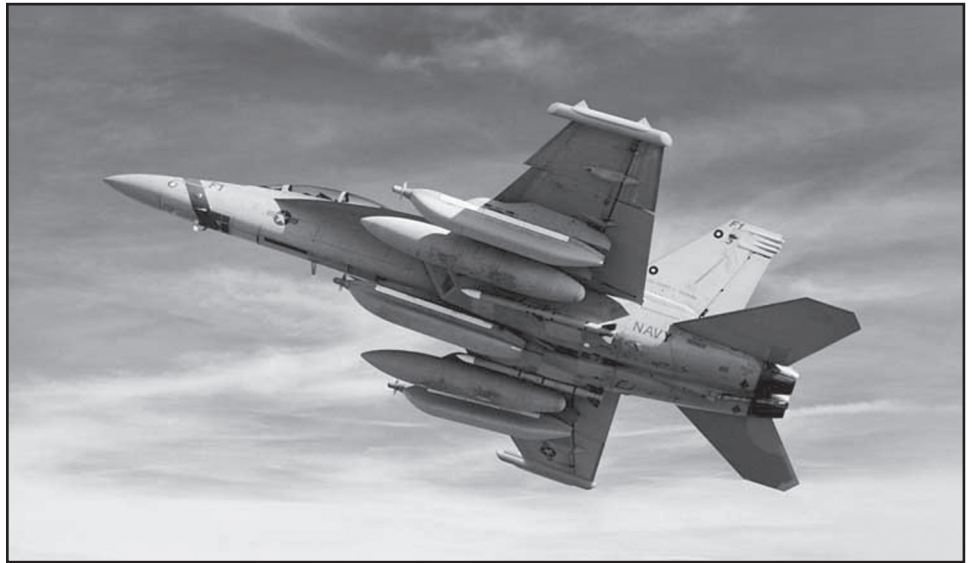
Figure 4: EA-18G Mock-up: F/A-18F Loaded with ALQ-99 Jamming Pods
