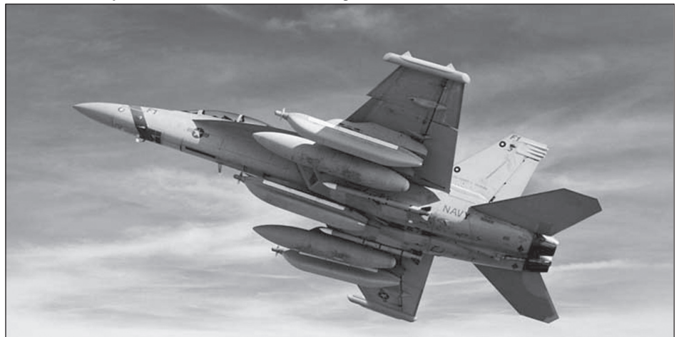
EA-18G Mockup: F/A-18F Loaded with Jamming Pods
