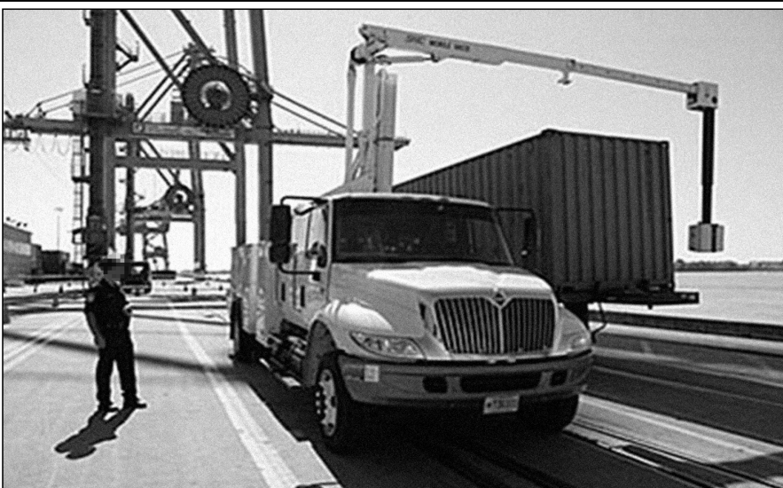
A truck X-ray machine in action.
