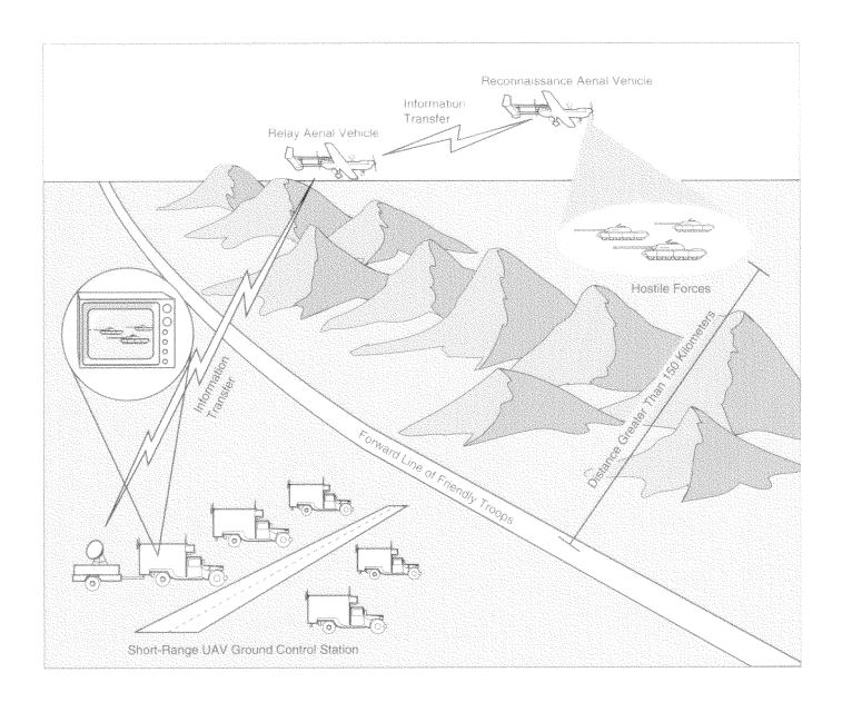
Most of the limited user tests planned to demonstrate this capability failed because of engine failures or other problems with the air vehicle and relay component. The test agency concluded that the system's ability to transmit
