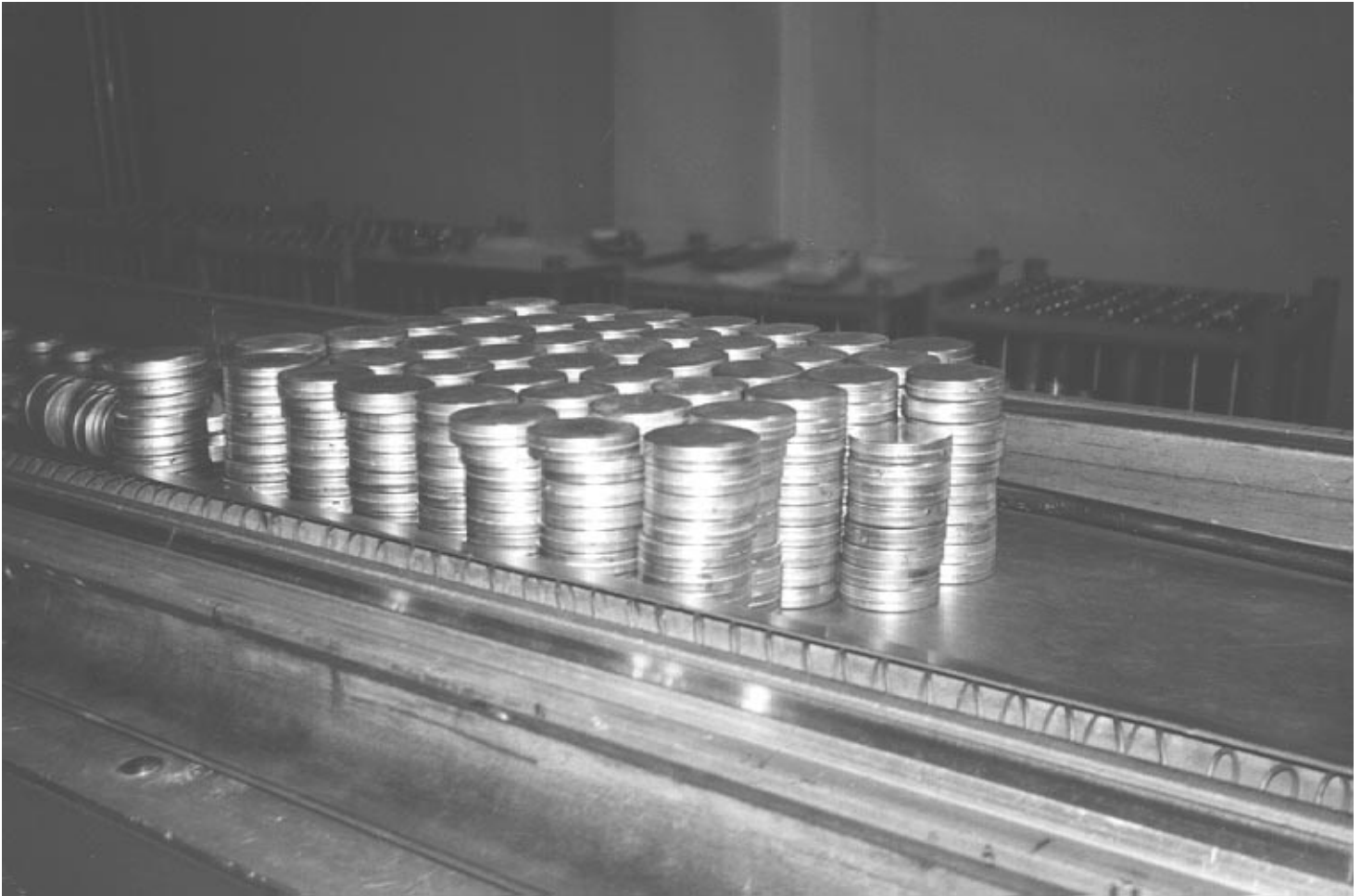
Figure 2.1: Examples of Small, Disk-Shaped Fuel Elements to Be Inventoried
