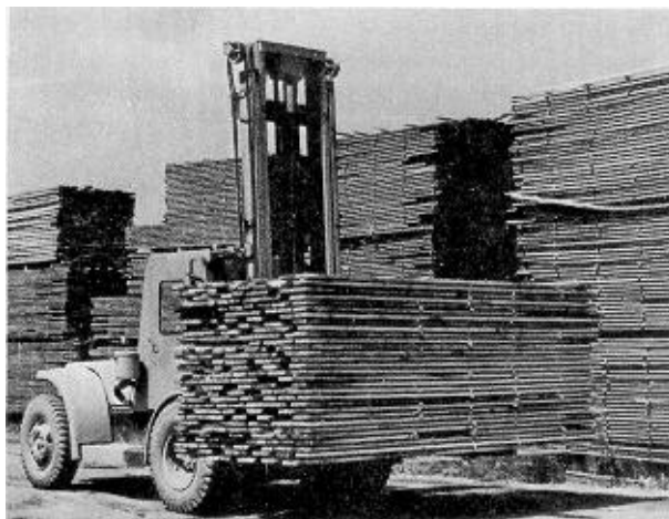
Figure 3.—Stacking stickered package of lumber.
