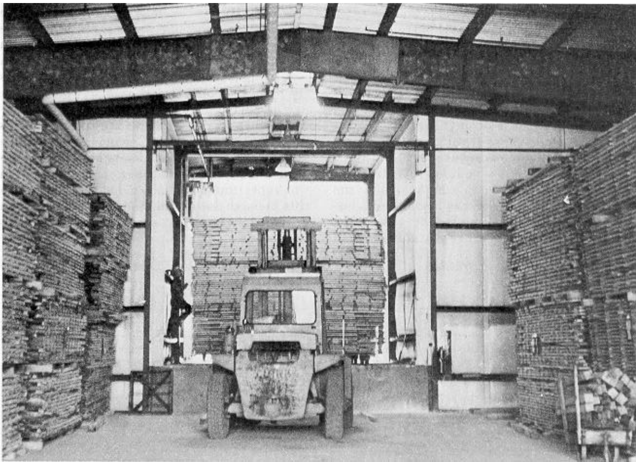
Figure 11.—Inside of a controlled-air dryer.
