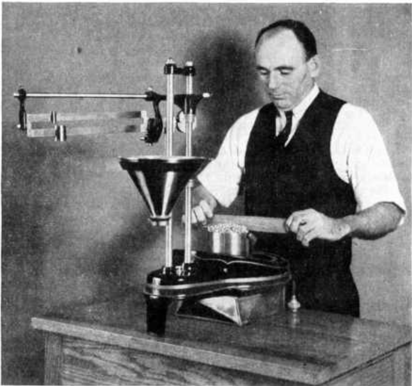
FIGURE 8.—Determining the test weight per bushel of grain in a grain inspection laboratory.
