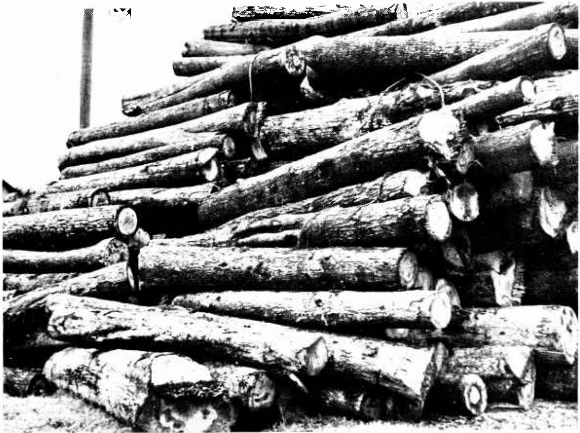
FIGURE 126.—Cold-decked logs. These logs are subject to checking and insect and fungus attack.
