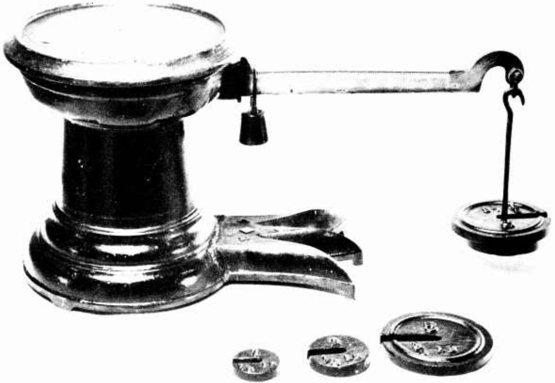
FIGURE 41.—Platform scale with capacity of 36 pounds and accuracy of 0.01 pound.
