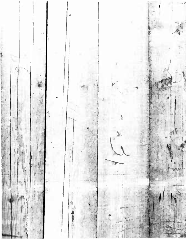
FIGURE 108.—Surface checking in Douglas-fir dimension lumber.
