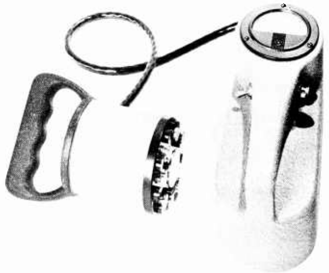
FIGURE 47.—A radio-frequency power-loss-type moisture meter.
