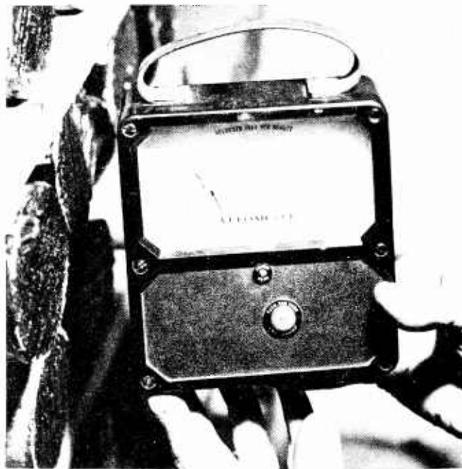
FIGURE 59.—A type of air velocity meter.
