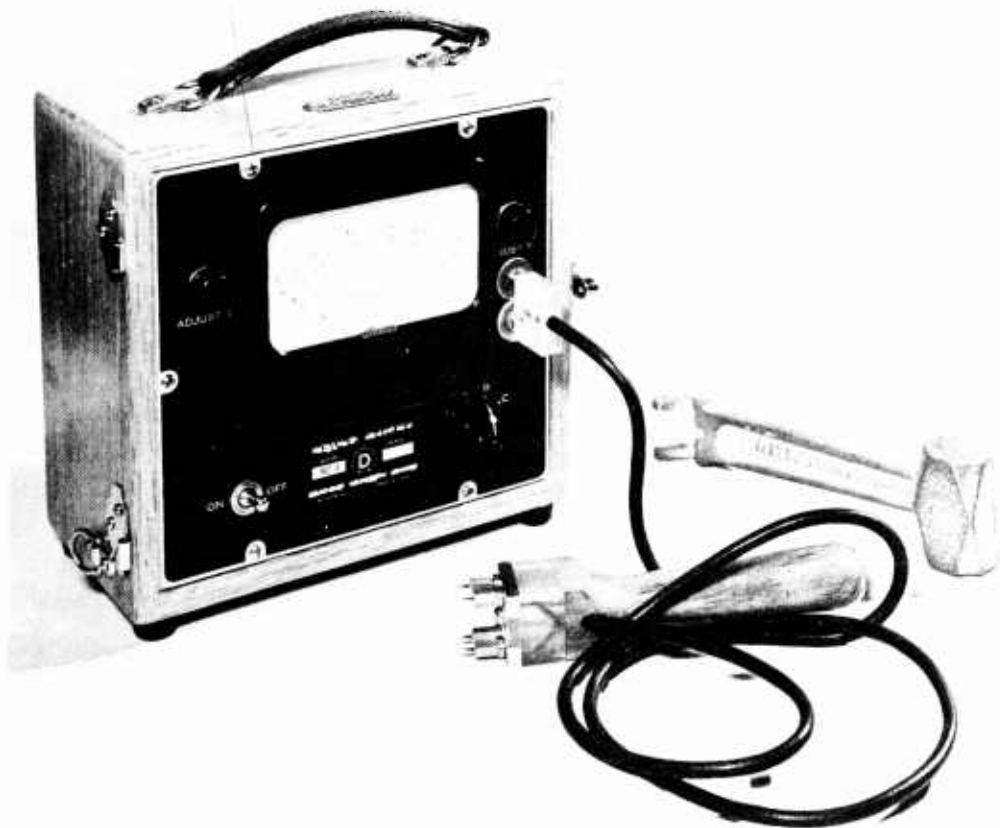
FIGURE 48.—A resistance-type moisture meter.
