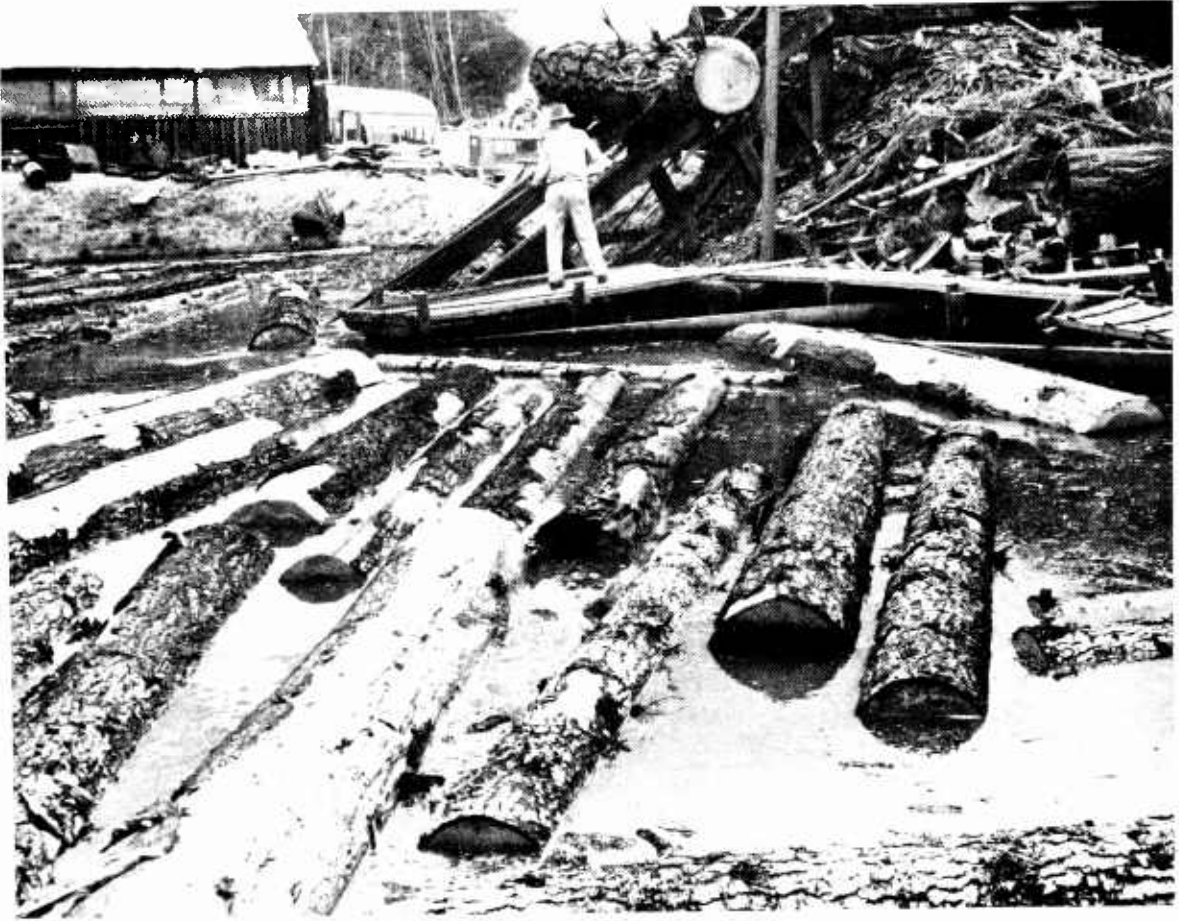
FIGURE 124.—Logs stored in a pond. Parts of the logs above the waterline may sustain drying defects and be attacked by insects and micro-organisms if stored too long in warm seasons.
