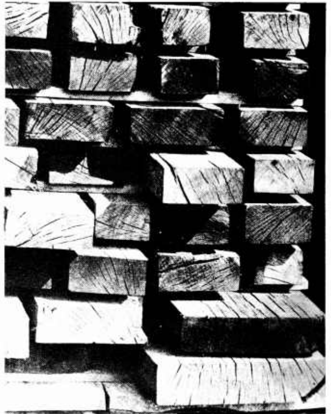
FIGURE 109.—End checks in oak plank.
