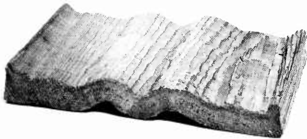
FIGURE 110.—Severe collapse in western redcedar.
