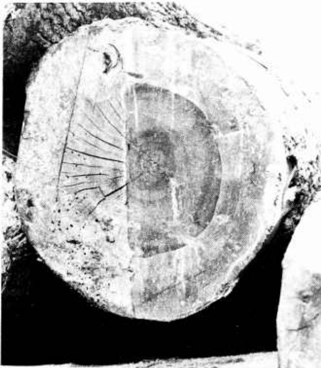
FIGURE 126.—Cold-decked logs. These logs are subject to checking and insect and fungus attack.
