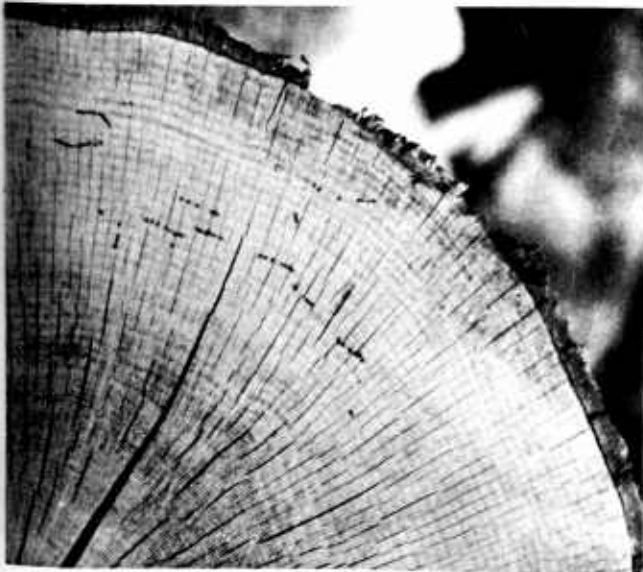
FIGURE 46.—Pin worm holes. F-455612
