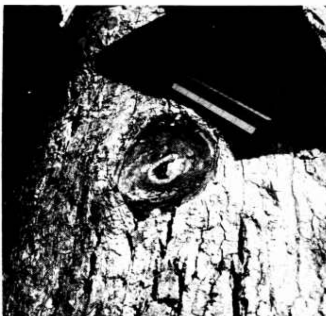
FIGURE 26.—Unsound log knot.
