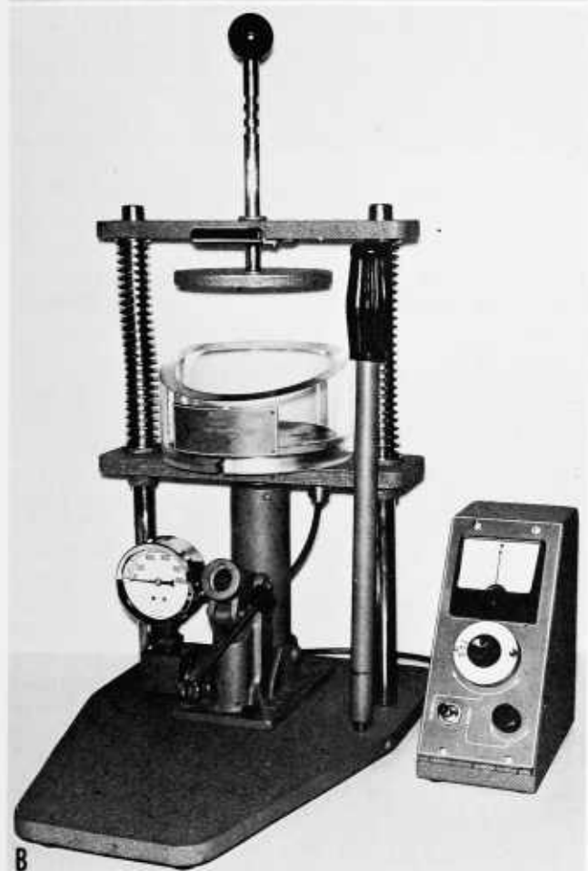
Figure 117. —Typical commercial line power-operated electrical resistance cotton moisture meters: A , an instrument with integral test chamber and indicator; and B , an instrument with separate sample test chamber and indicator.
