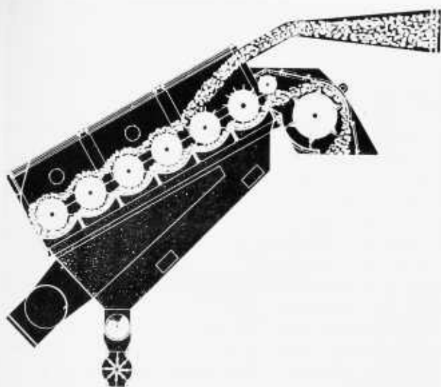
Figure 37.—Cross section showing flow of cotton through an inclined cleaner.
