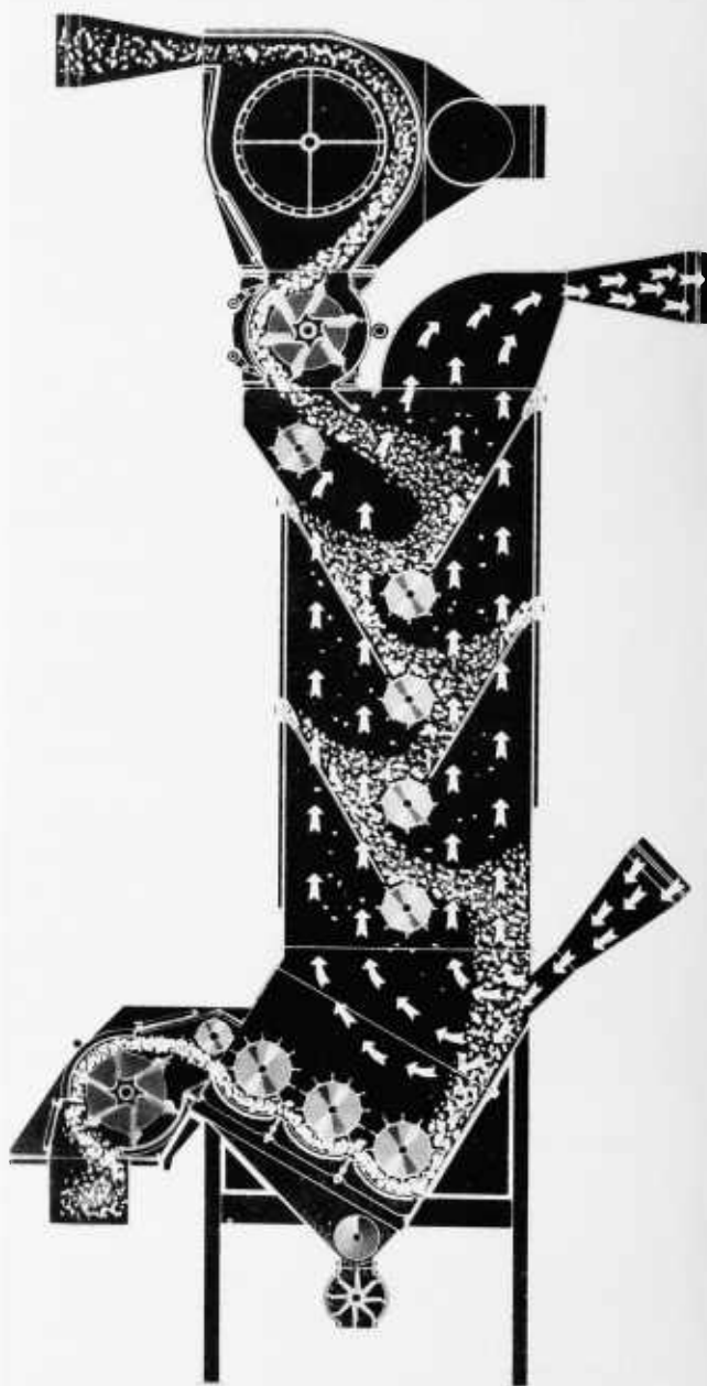
Figure 20.—Cross section of a vertical counterflow-type seed cotton drier incorporating seed cotton cleaning apparatus.
