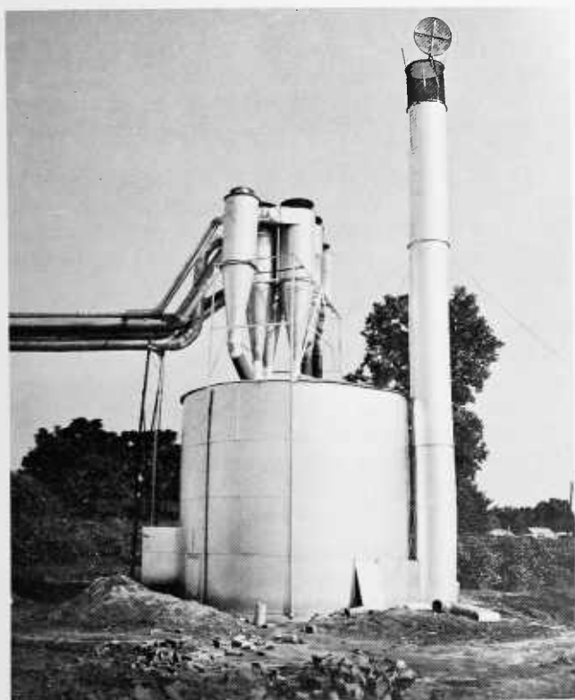
Figure 110.—Incinerator with small-diameter cyclones on top in use near Stoneville, Miss.
