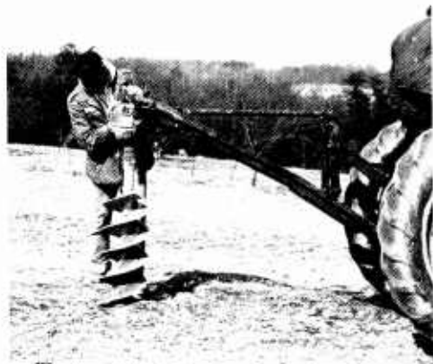
FIGURE 5.—Hole-digging auger used for tree planting. Power is from the takeoff on the tractor.
