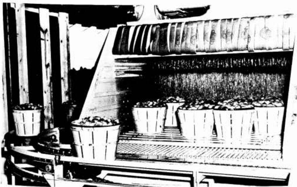
FIGURE 27.—Typical peach hydrocooler in operation. (Courtesy of Food Machinery and Chemical Corporation, Lakeland, Fla.)
