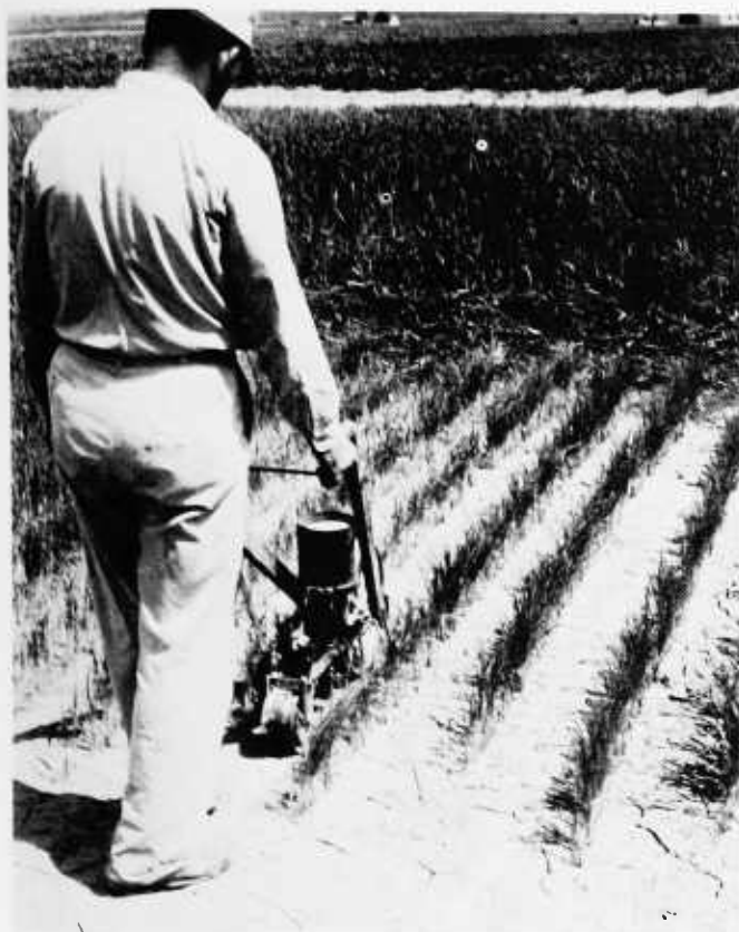
FIGURE 11.—A distributor used to apply nitrogen fertilizer between the rows as a topdressing.
