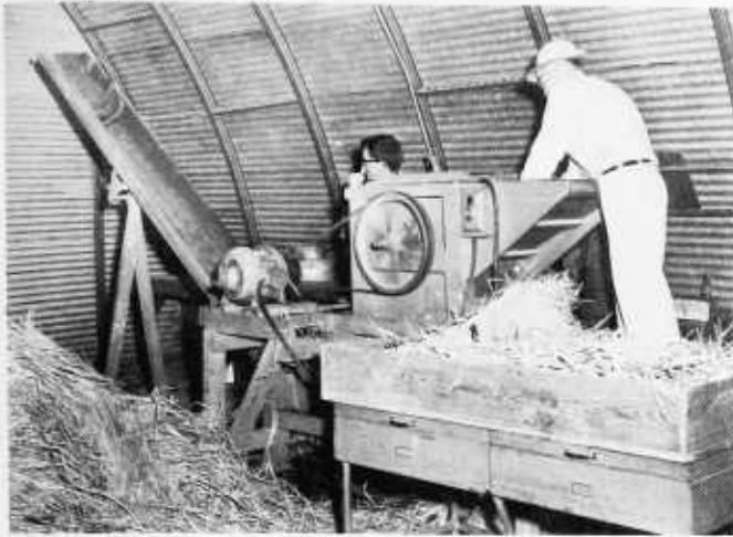
FIGURE 15.—Threshing bundles of rice from nursery yield experiment with a modified Kansas nursery thresher.
