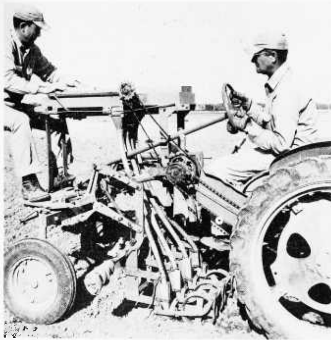
FIGURE 9.—Belt seeder, mounted on a small tractor, used for seeding nursery yield experiments.
