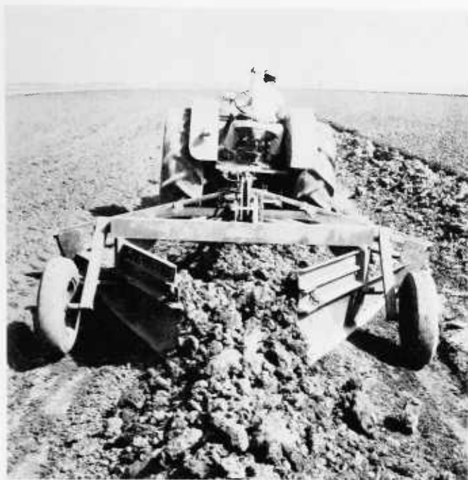
FIGURE 7.—Constructing levees in the nursery with a steel-bladed levee builder.
