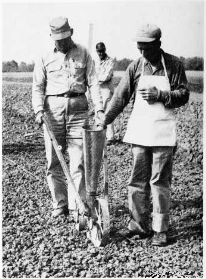
FIGURE 10.—Manually operated seeder used to seed selections.
