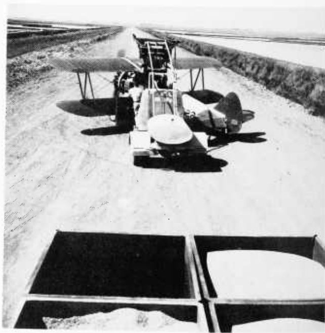
FIGURE 33.—Airplane being loaded with seed rice, with tanks used for soaking seed in the foreground, and ricefields ready to be seeded on each side of landing strip.
