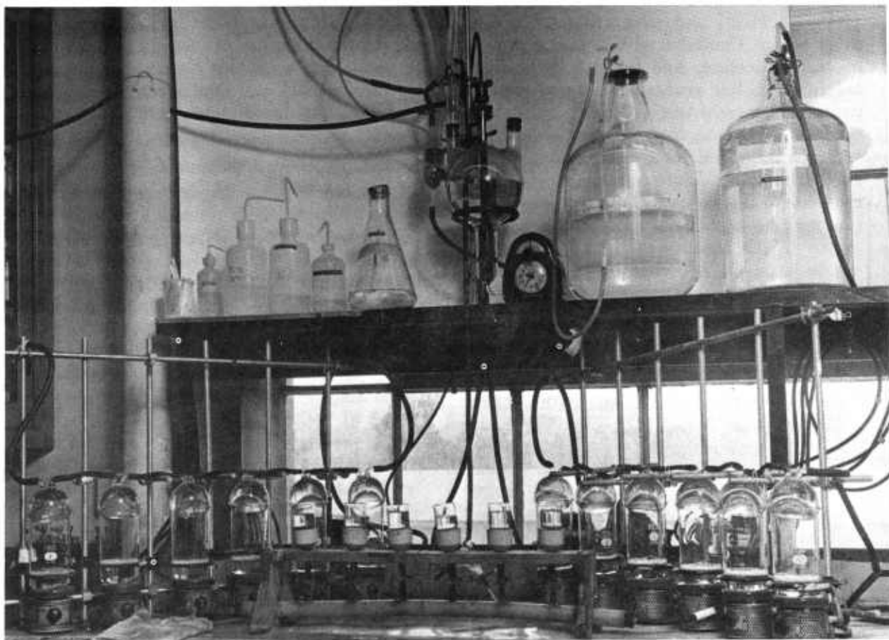
FIGURE 7.—Assembly of 12 units of refluxing apparatus with filter manifold and hot-water system.
