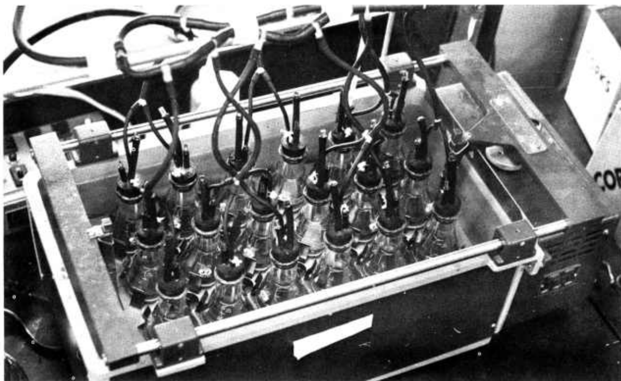
FIGURE 8.—Arrangement of water bath for in vitro fermentations.
