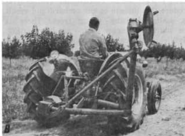
FIGURE 10.—Tractor-mounted rotary tree hoes: A, Drum-type with optional rotovator blades and depth-controlling wheel; B, floating-head type with the shaft lifted into road position.
