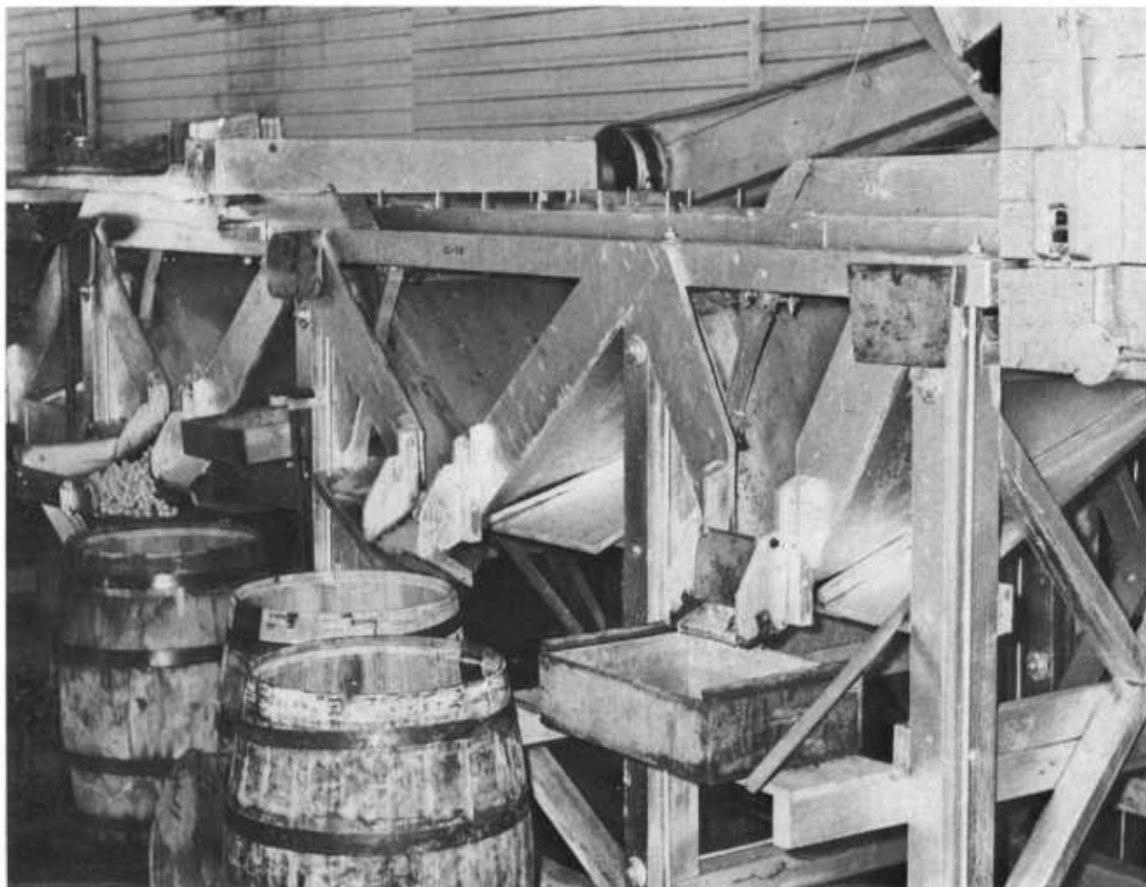
FIGURE 65.—Size-grader. Brined cherries are graded for size over vibrating perforated screens. Graded cherries are discharged through separate chutes.
