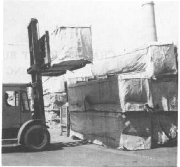
Figure 57.—Forklift truck removes a wrapped package of lumber to be used at a manufacturing facility.
