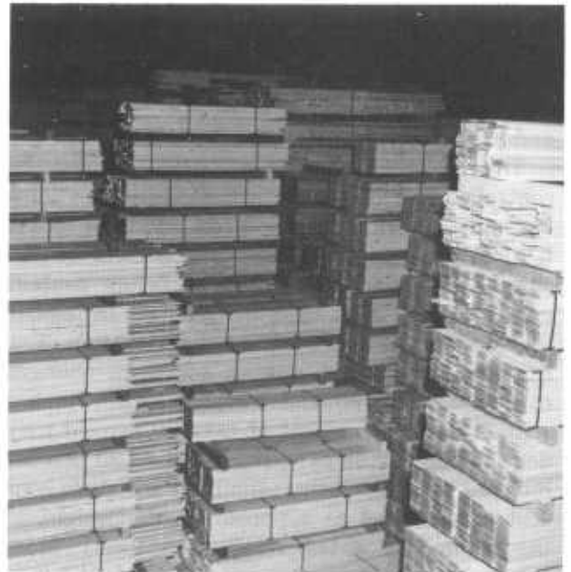
Figure 3.—Kiln-dried, finished softwood lumber stored in a large closed shed. The strapped packages are transported by an overhead gantry crane.
