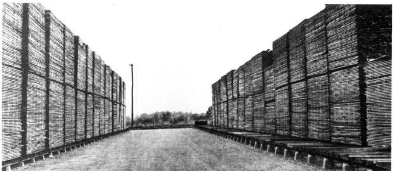
Figure 20.—Stickered unit packages of hardwood lumber piled on permanent foundations in a “line-type” forklift yard.
