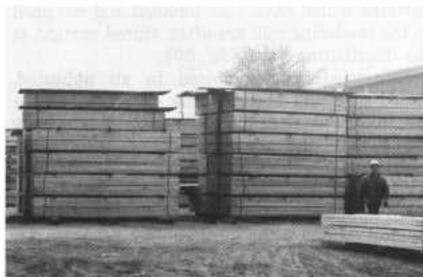
Figure 45.—Outdoor storage of dry, finished softwood lumber. Note the use of pile roofs to provide some protection from rain and sun.
