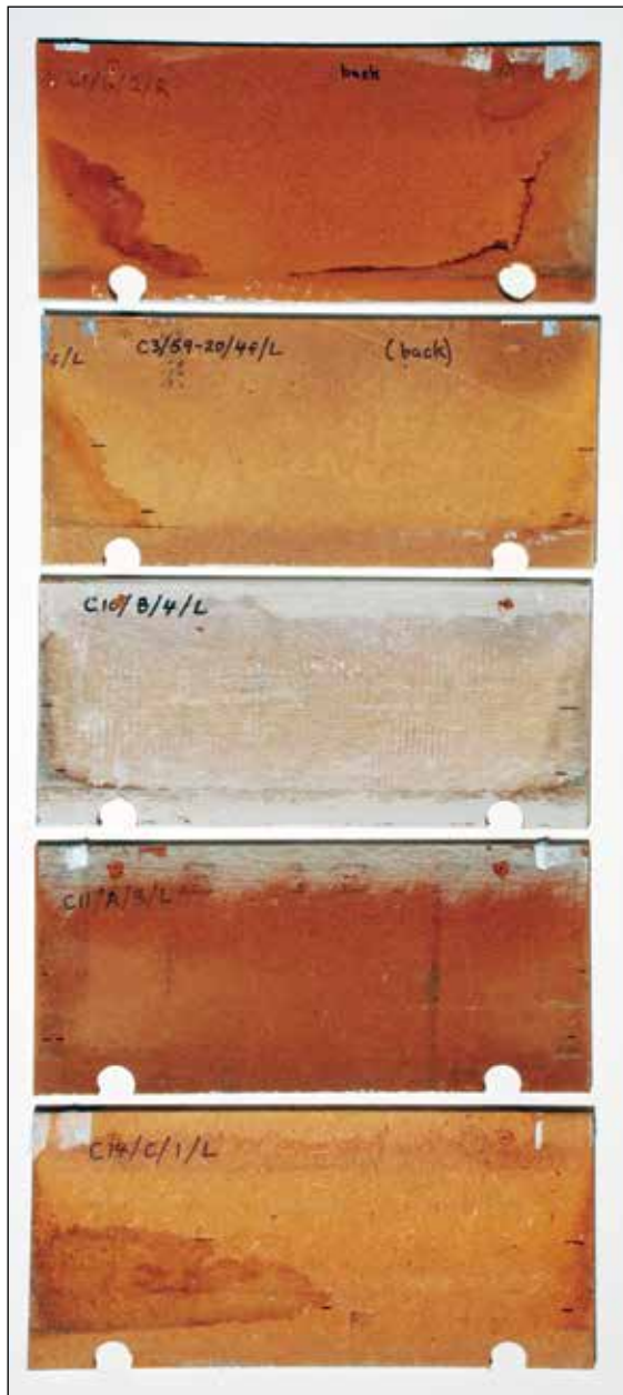
Figure 4. Rear surfaces of five specimens with staining wholly or mostly restricted to areas above the lap. In specimen C11/A/3/L, the extent of staining is modest, and the intensity so modest as to be barely perceptible. With the exception of specimen C14/C/1/L, these specimens had more extensive staining than average for their respective board classes.
