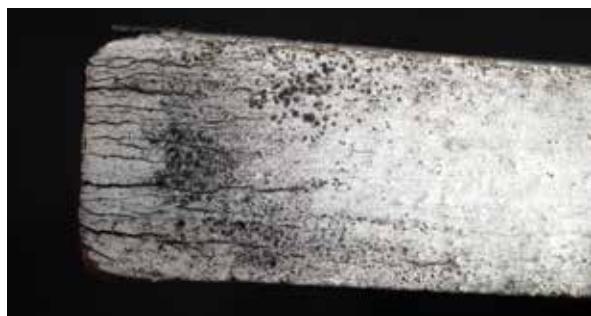
Figure 7a. Magnified image of the end of the drip edge of a specimen of Class 1 board. Drip-edge paint cracking is prevalent near the end of the specimen, but does not extend more than 16 mm from the specimen end. Patches of mildew are present only near the inboard terminations of drip-edge cracks. This specimen was from a bottom course location, (where water exposure was greatest), and in the left-most column of specimens (at the southwest corner of the building). This specimen showed more drip-edge mildew than any other specimen. In this photograph the outer specimen face is at the top of the specimen.
