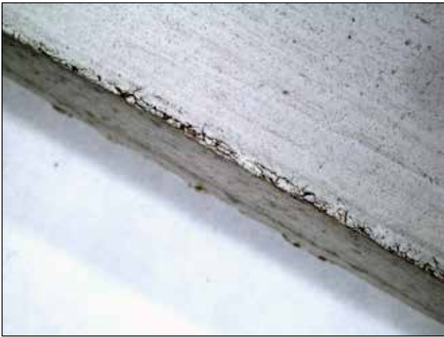
Figure 12. Magnified image showing initiation of cracking at the interface of the drip edge and the outer specimen face in a specimen of class 2 board. With the exception of these observed cracks, some cracking near the unpainted end cuts, and some surface dirt, the specimen was in pristine condition after 155 months of exposure. This specimen did not have a shaped drip edge, inasmuch as it was a specimen of noncommercial board.
