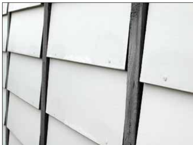
Figure 2. Two adjacent specimens in a column, each showing edge welting. This photo was taken after roughly 7 years of exposure. Welting is predominantly at mid-length of specimen (between the nails). Note lack of perceptible swelling (or welting) at the nails. The points at which on-fence thickness was measured were slightly outboard of (toward specimens ends from) the nails.
