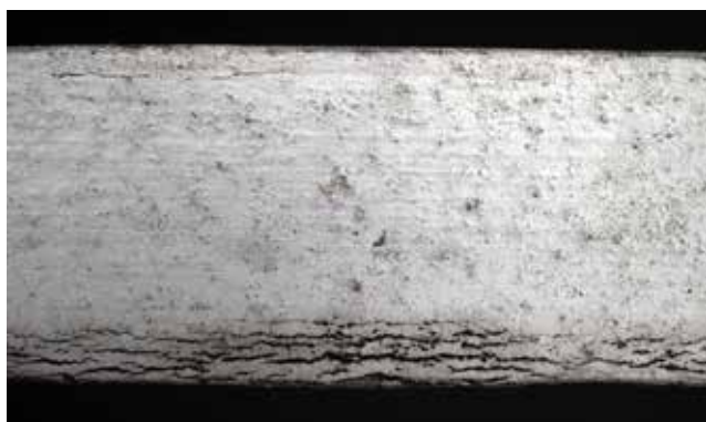
Figure 7b. Magnified image of the drip edge of a specimen of class 4 board approximately at specimen mid-length. A patch of drip-edge cracks is present near the outer edge of the drip edge, and a small amount of mildew is present in the patch of drip-edge cracks. The specimen was from a bottom course location. In this photograph, the outer specimen face is at the bottom of the specimen.
