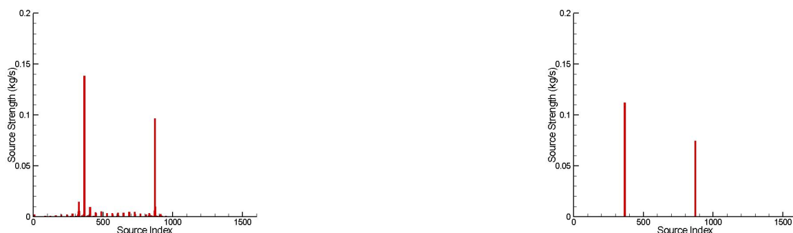
Figure 19: Results of the bootstrap procedure when noisy measurement data from two different wind directions are used in a single inversion procedure. The left sub-figure shows a bar plot of the maximum predicted values over 1000 iterations, while the right sub-figure shows a bar plot of the minimum values.
