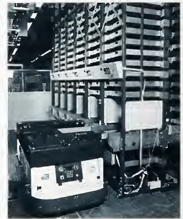
Fig. 10 The "racker stacker" stored about a week's worth of blanks, tools, and other pieces needed by the individual AMRF workstations. (Photo collection, AMRF Files, NIST)
