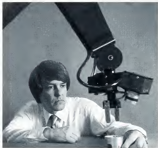
Figure 12. James Albus pioneered the idea of structured light for guiding a robot vision system. (Photo collection, ISD, NIST)
