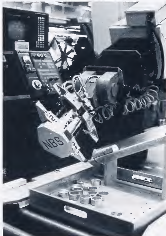
Figure 1. The robot arm of the Turning Workstation (TWS) swings into action to pick up the finished product from the turning center machine tool. (Photo collection, AMRF Files, NIST)
