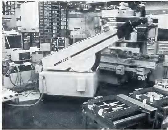
Figure 6. The Unimate 4000 robot loaded blanks into the Monarch VMC 75 computer numerical control (CNC) vertical spindle machining center. A pioneering automated process planning system generated the numerical code, verified it, and directed the machining center to cut the part as designed by the user, totally hands off. (Photo collection, AMRF Files, NIST)
